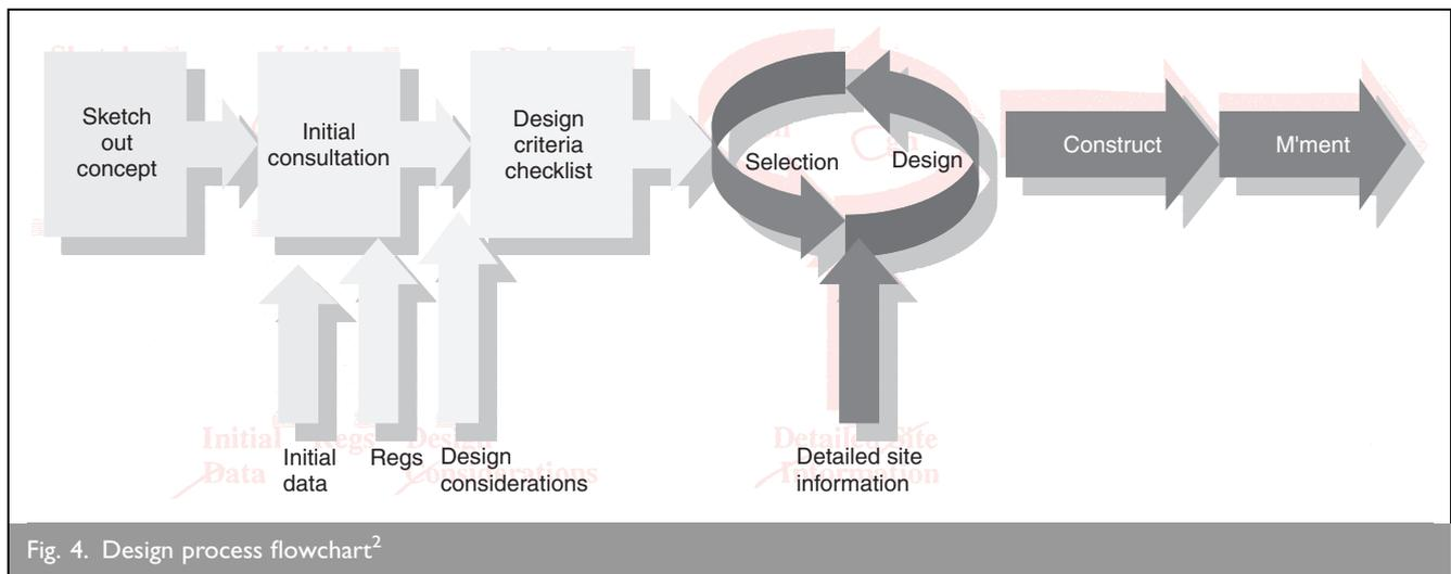
Fig. 4. Design process flowchart<sup>2</sup>
