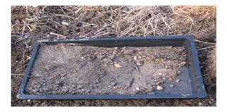
The silt trap works by slowing the flow of water, allowing soil particles and attached nutrients or pesticides to filter out. A tray placed at the bottom of the silt trap in December 2009 demonstrates the amount of material collected in just one month and after 52 mm of rainfall. Amongst the sediment was an abundance of fresh water invertebrates.
