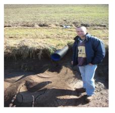
The picture shows the amount of soil collected over the course of one month that would have otherwise entered the surface water network. The water collected slowly drains
